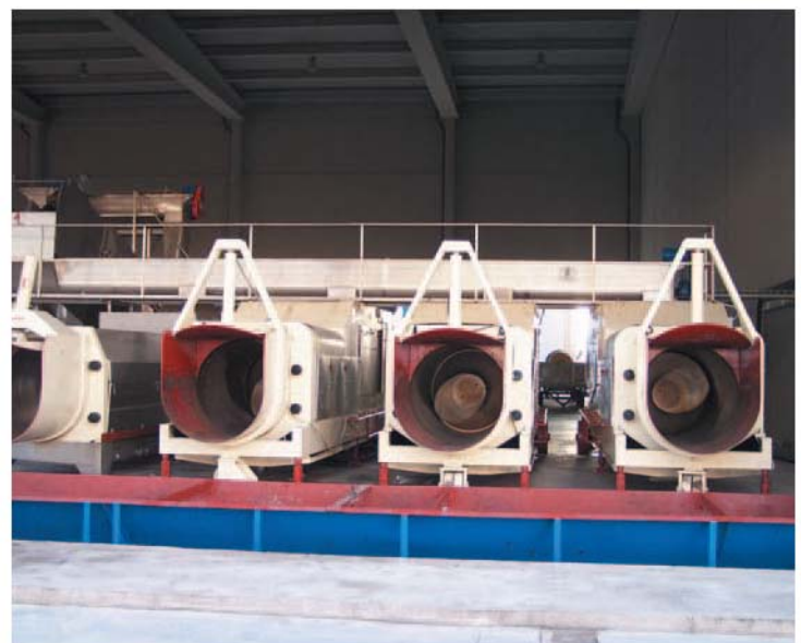
Continuous presses apply aggressive pressing
