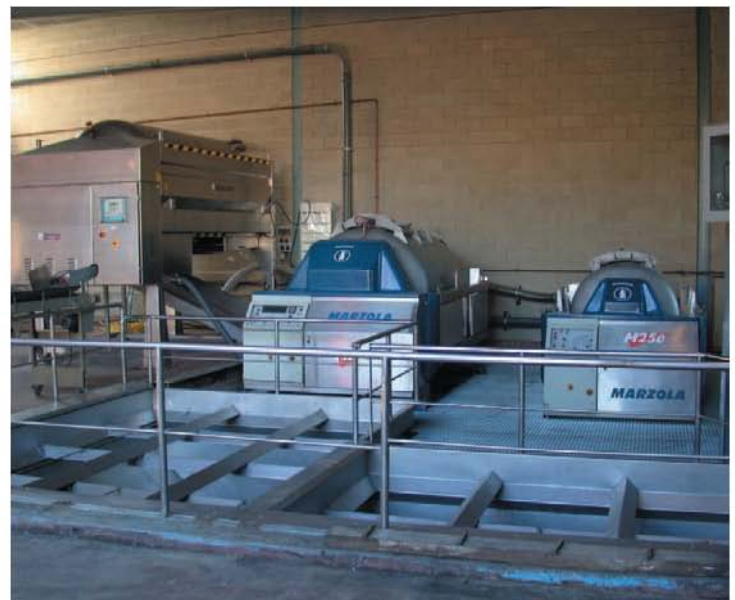
Pneumatic presses favour a soft and adequate pressing
